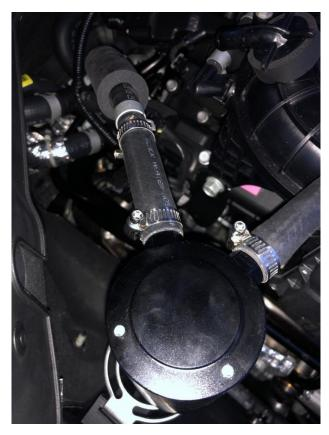
9. Locate the two extruding bolts to attach bracket
